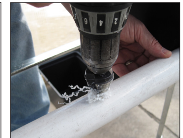
Photo shows using a step bit to drill holes in the pvc pipe.
