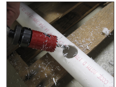
Photo shows using a hole saw bit to drill holes in pvc pipe.
