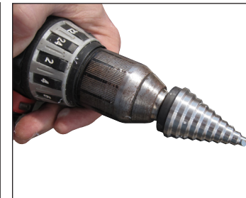
Photo shows using a step bit to drill holes in the pvc pipe.
