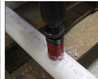
Photo shows using a hole saw bit to drill holes in pvc pipe.
