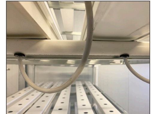
c. Slide one tube into each of the supply manifold grommets.
