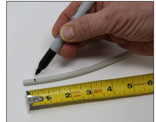
b. Mark tube for depth of insertion into grommet.
