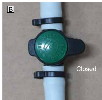
3/4" hose connected to AC2804 in-line valve. Install one valve in each riser. Make sure the 111698 clamps do not interfere with valve operation.
