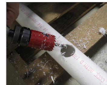
Photo shows using a hole saw bit to drill holes in pvc pipe.
