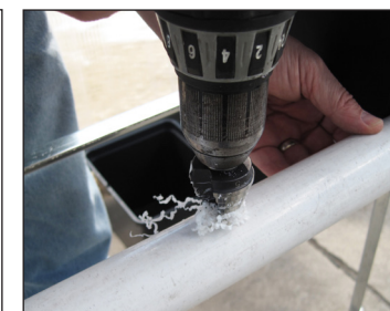
Photo shows using a step bit to drill holes in the pvc pipe.
