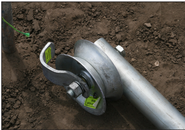
111931 Castor with safety guard, mounting bolt, lock washer, & nut
