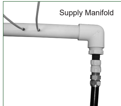
STEP 3: Disconnect hose here if using supply hose to drain reservoir. If you are using a different hose to drain reservoir, disconnect supply hose from pump fitting and connect customer-supplied drain hose. Ball valve is shown in the closed position.
