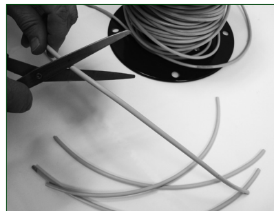
1. Cut the 12" supply tubes from the 111046 poly tubing
