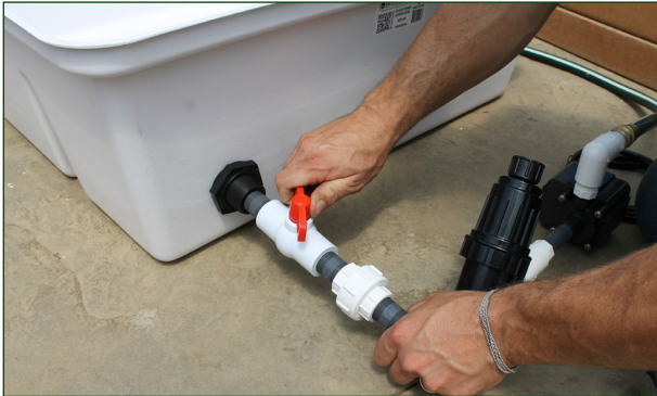
STEP 2: With the pump off, close ball valve.
