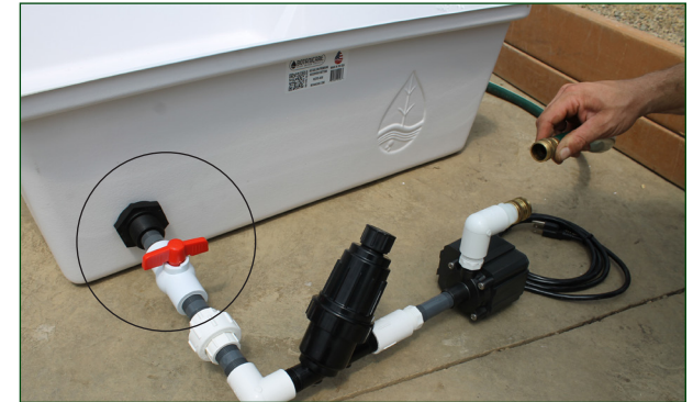
STEP 3: Disconnect hose here if using supply hose to drain reservoir. If you are using a different hose to drain reservoir, disconnect supply hose from pump fitting and connect customer-supplied drain hose. Ball valve is shown in the closed position.
