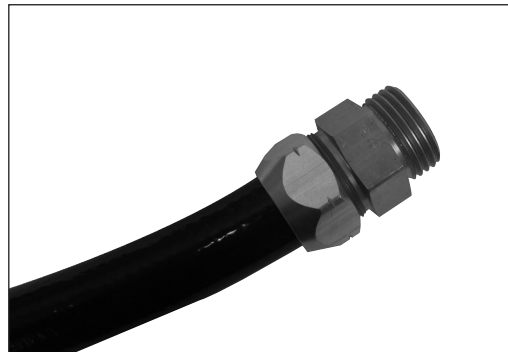
5. Completed male fitting end.
