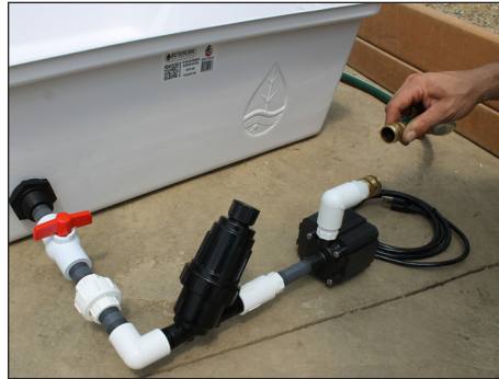
STEP 3: Remove supply hose from pump fitting assembly.
