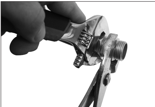
4. Start collar onto the fitting treads and tighten.
