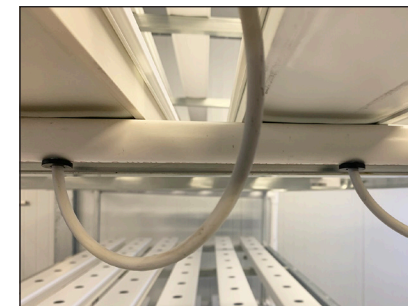
2. Slide one tube onto each of the supply manifold 115820 grommets.
