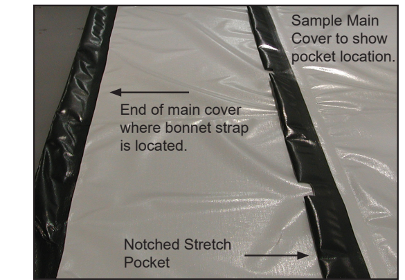
Photo above shows a similar cover and the location of the stretch pocket. Cover is shown with the underside facing up, which is the side visible from inside the frame when the cover is installed.
