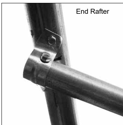
The above photo shows how to secure the angled purlin to the underside of the assembled rafters and frame. Use FA4482B Tek screws and QH1070 pipe straps.
