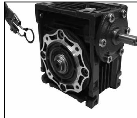
Using a snap ring pliers, place snap ring over shaft and seat into machined groove on shaft.
