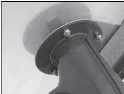
Inside view showing fan mounting bracket and the mounting bolts for the fan.
