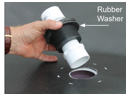
l. Slide rubber washer over fitting threads and insert assembly through liner.
