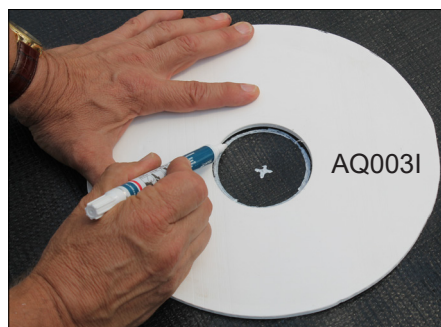
e. Use washer as a template to mark fitting position.
