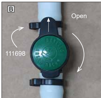
3/4" hose connected to AC2804 in-line valve. Install one valve in each riser. Make sure the 111698 clamps do not interfere with valve operation.
