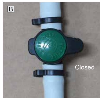
3/4" hose connected to AC2804 in-line valve. Install one valve in each riser. Make sure the 111698 clamps do not interfere with valve operation.
