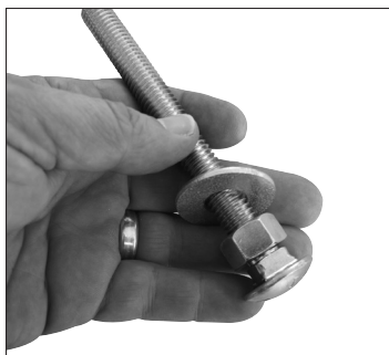
FIGURE 1: Assemble levelers as shown.
