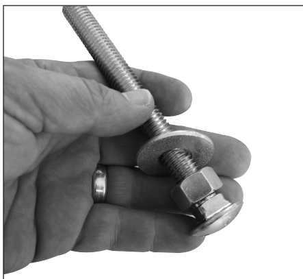
FIGURE 1: Assemble levelers as shown.
