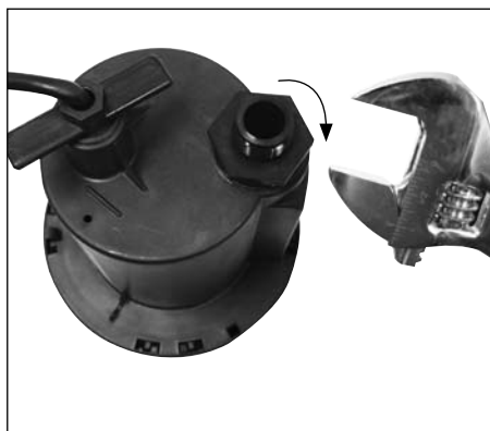
2. Tighten fitting until snug. To prevent damage to the pump housing, do not overtighten.
