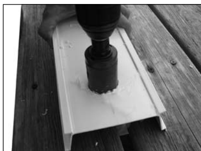
Drill holes in channel bottom.
