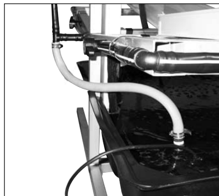
7. Set the pump in the reservoir. Keep the power cord outside the reservoir.
