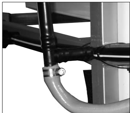
5. Attach the free end of the hose to the T-fitting at the lower end of the Riser Assembly.
