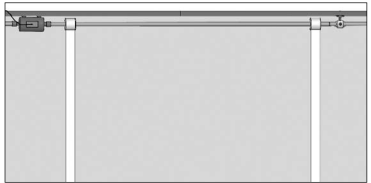
Drawing shows the electric roll-up room divider installed within a framed opening. Panel and straps are installed later.
