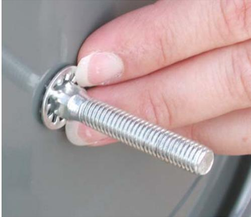
7. Add the spacer, align the holes in the support frame, and insert the bolt assembly through the holes in the support frame.
