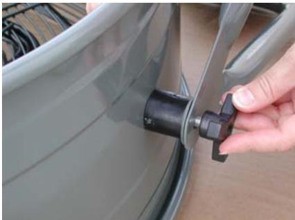
9. After securing the support frame to the main fan housing, recheck the handle mounting bolts to verify that they are tight.
