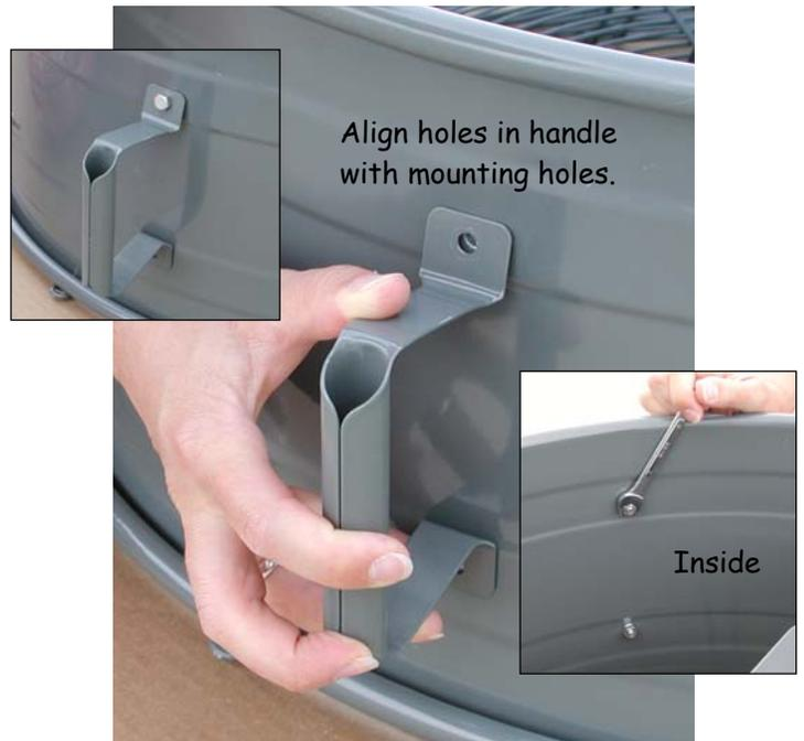
Insert bolts from the outside and install the flat washer, lock washer and nut on the inside of the main housing as shown. Tighten bolts using a wrench.
