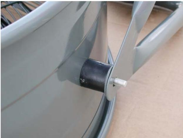
8. Add the adjusting knob and repeat the steps to attach the remaining side of the support frame to the main fan housing.
