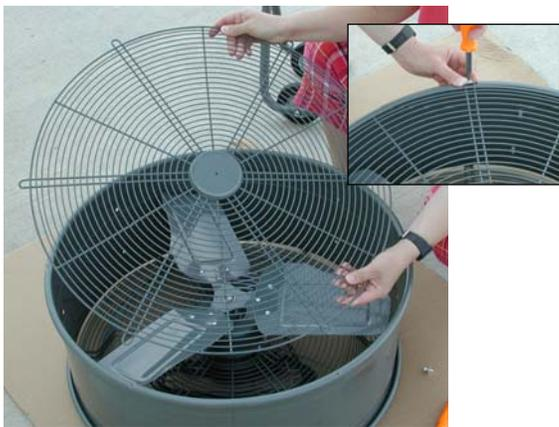
Position motor side down and the fan up as shown. Cardboard is used to protect the finish.
