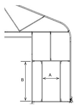
**NOTE:** The 1.50" square tubing or a wood 2 x 4 will not fit into the door jamb channel. The rough opening must be larger than the door jamb outside dimensions.
