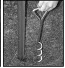
STEP 3: Twist stake clockwise until triangular top touches the ground.
