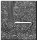
STEP 4: Secure long strap and attached S-Hook to the coupler.
